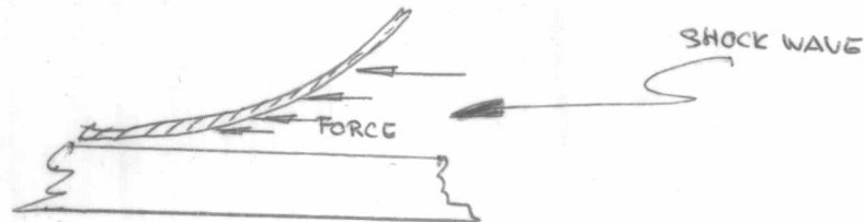
Fig. 8 Shock Wave Shearing Metal.
