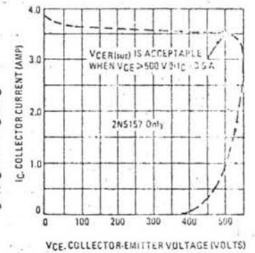
FIGURE 12 - COLLECTOR-EMITTER SUSTAINING VOLTAGE TEST CIRCUITS AND LOAD LINES
