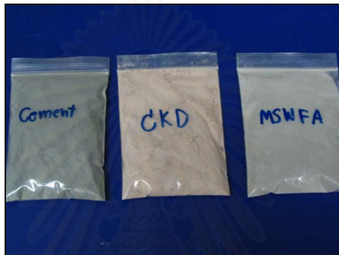
Figure 3.7 Cement, cement kiln dust (CKD), and municipal solid waste fly ash (MSWFA).
