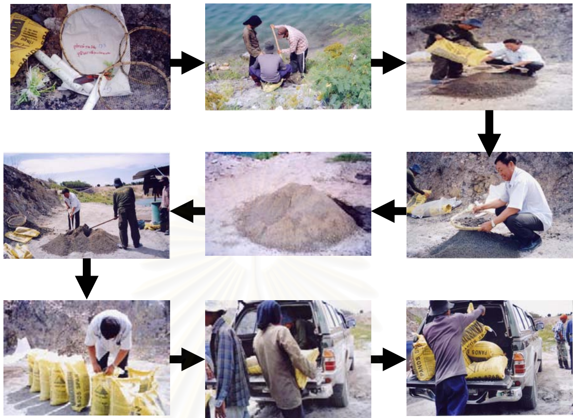
FigureA-2 Steps of soil sampling in site
