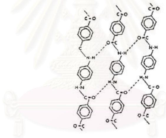
Figure 2.2 Chemical structure of Kevlar [9].
