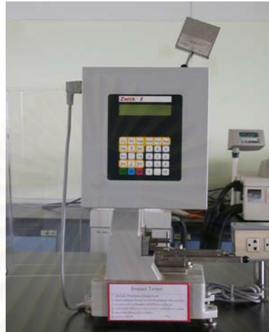
Figure 3.13 A Zwick 5102 Pendulum impact tester (Izod-type)
