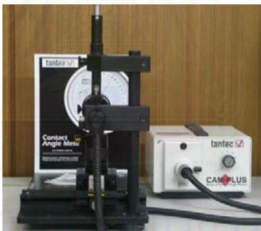
Figure 3.6 Cam-Plus Tantac contact angle meter
