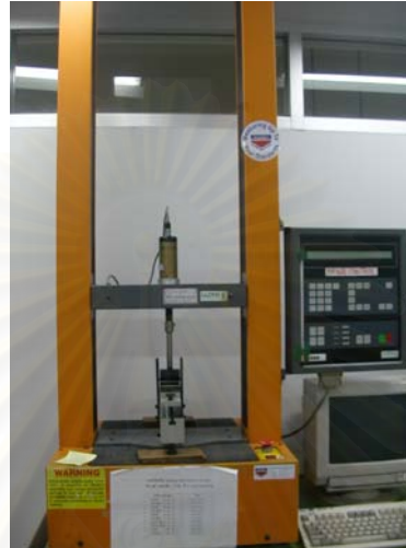
Figure 3.11 A LLOYD Universal testing machine model 500
