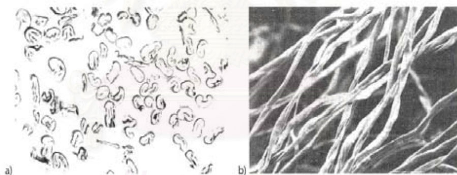
Figure 2.3 Cotton fibers [12]. (a) Cross-section
