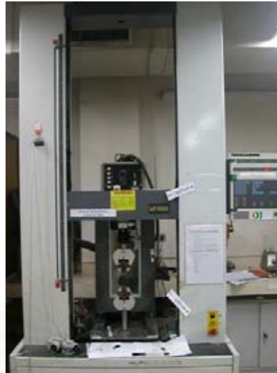
Figure 3.9 A LLOYD Universal testing machine model LR 100K
