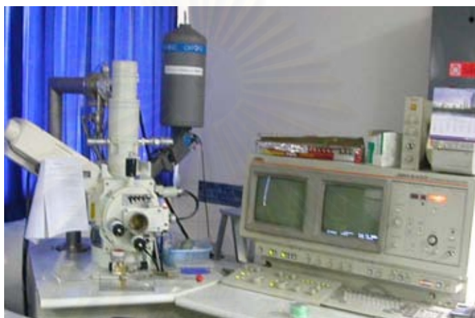
Figure 3.15 A Joel JSM-6400 scanning electron microscope
