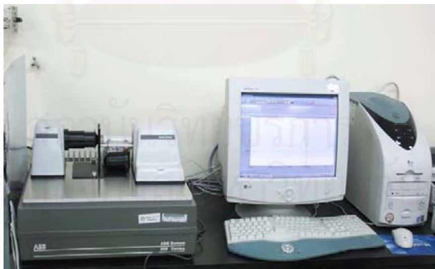
Figure 3.7 Attenuated total reflection/fourier transform infrared spectroscopy
