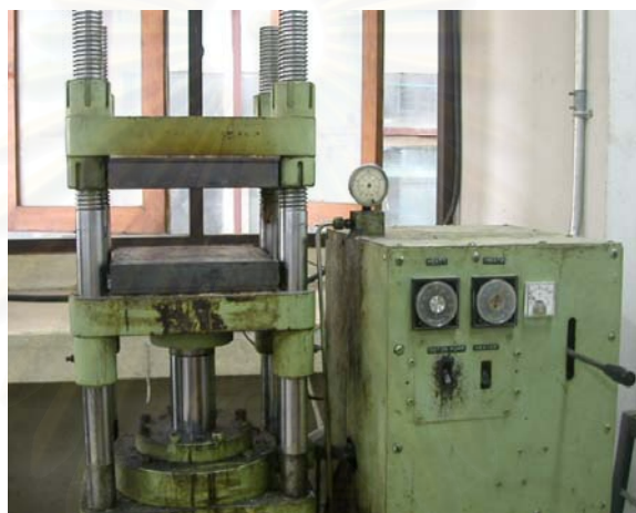
Figure 3.8 Compression molding machine
