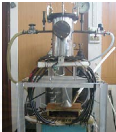
Figure 3.4 UNU/ICTP plasma focus device
