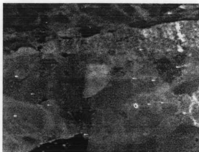
(a) Cross sectional micrograph of oxide film
