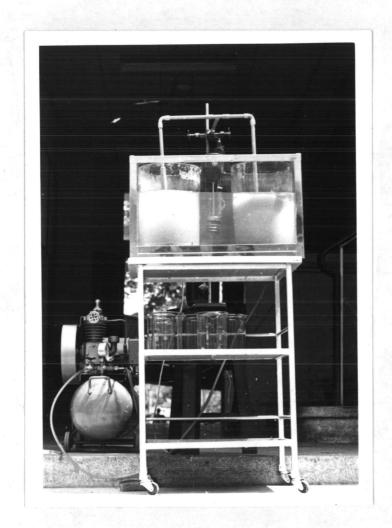
FIG. 7 THE LABORATORY-SCALE AEROBIC DIGESTION SET-UP
