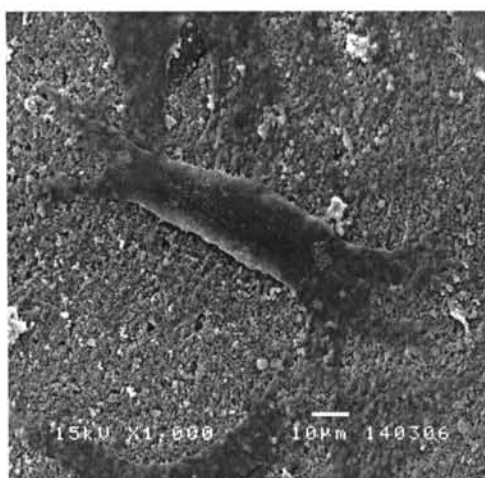
Figure 10 Scanning electron micrograph of HPDLs attached to Tetric ® Flow at 24-hour incubation. (central area) (original magnification x1000).
