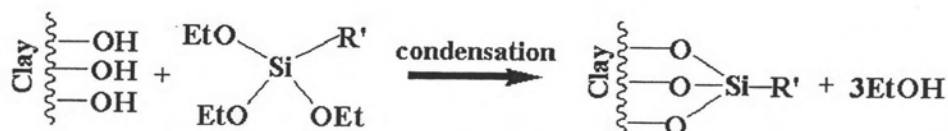
Scheme 2.1 The reaction of alkoxy groups of organosilane with the silanol groups on the clay surface.
