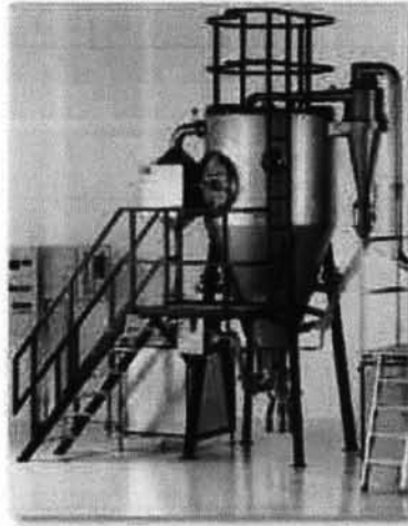
Figure 2.1: Spray dryer, a type of liquid drying
