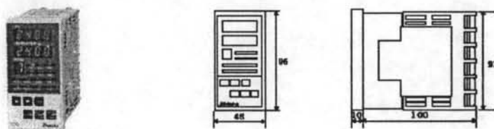
Figure 3.2 Microcomputer Based Temperature Indicating Controller FCR-13A
