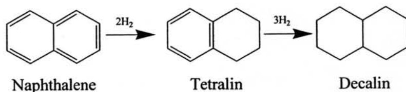
Figure 1.1 Sequential hydrogenation reaction of naphthalene.
