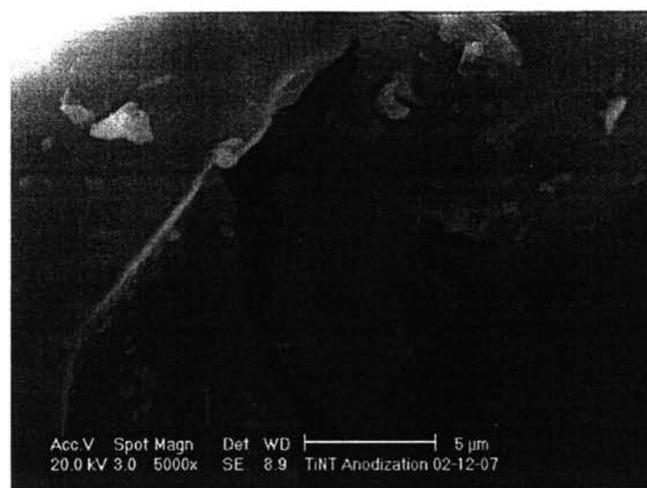
Figure B3 SEM micrograph of analcime particles partially dissolved in sulfuric acid and coexisting with the precipitate.
