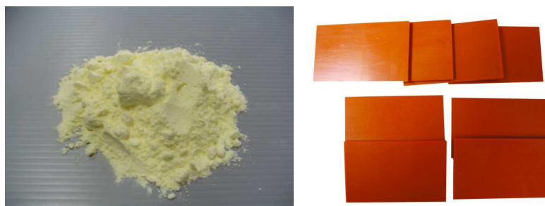
Figure 2.13 Benzoxazine resin powders and molding. [12]
