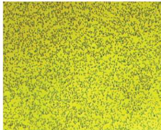
Figure 3.4 Microstructure of modified asphalt by epoxy resin. [14]
