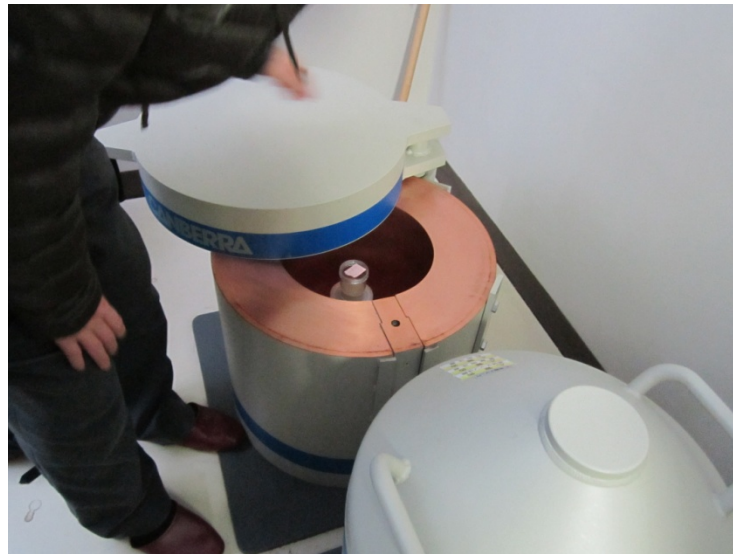
Figure 2.20 Gamma ray spectrometer at Akita University, Japan. This equipment is used for measure uranium, thorium and potassium contents.
