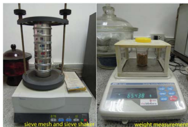
Figure 2.8 Photographs showing sieve mesh and sieve shaker and weight measurement used in this study.
