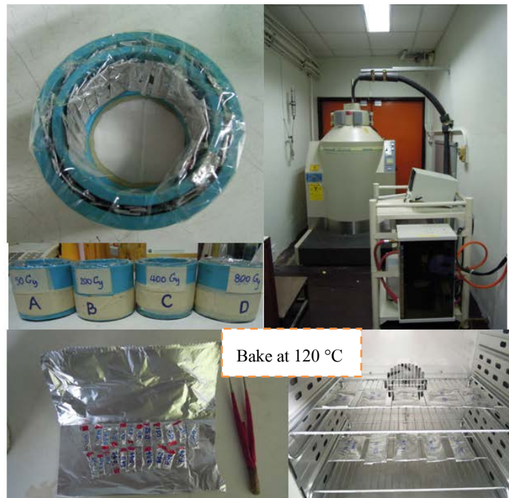
Figure 2.24 Sample for irradiation by Gamma cell (Source ^{60}\text{Co} ) at 50Gy, 200Gy 400Gy and 800Gy at Office of Atoms for Peace. After that baked it at 120 °C (1 day) for reduce noise.
