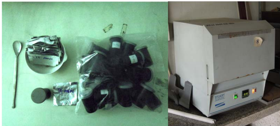
Figure 2.22 Sample is brought into Aluminium foil and baked it at 320 °C around 5 hours for reset electron to zero.
