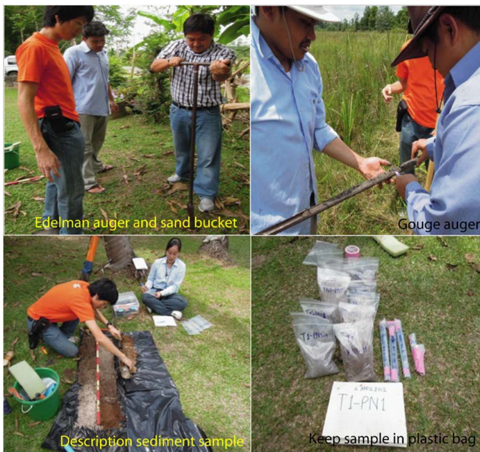
Figure 2.3 Field measurement for sampling sediments. (top left) hand auger; Edelman auger and sand bucket (sampling sand), (top right) gouge auger (sampling mud). (bottom left) description of samples and (bottom right) samples were kept from each 20 centimeter depth in zip-lock plastic bag.
