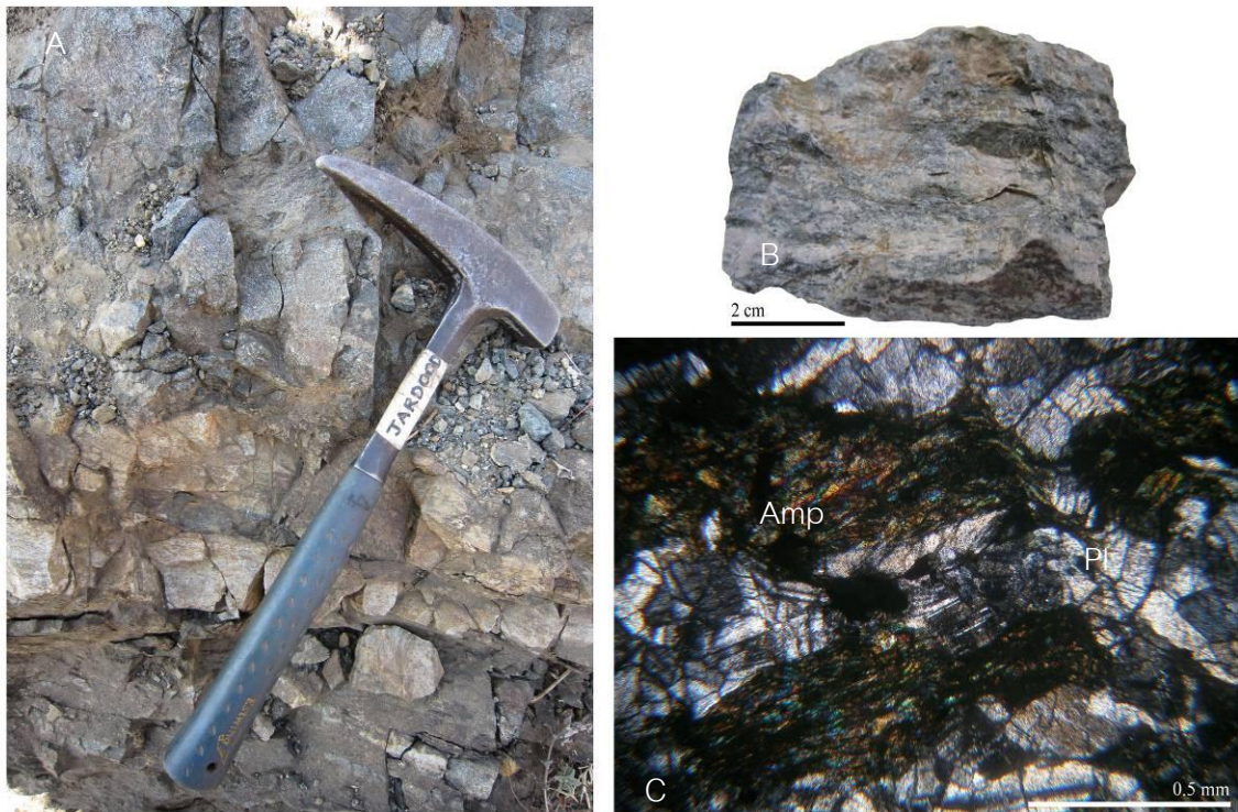
Figure 3.8. Layered amphibolites: A) an outcrop showing clearly layers between black greenish minerals (amphibole) and white minerals (mostly plagioclase) that is typical feature of this rock group; B) a hand specimen presenting the layers of minerals; C) photomicrograph showing the layers between amphibole (Amp) and plagioclase (Pl) under cross-polarized (XPL)
