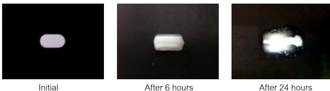
Figure 31 The physical appearance of multilayer sustained release tablets of sodium valproate combined with valproic acid after exposed to dissolution medium at 0, 6 and 24 hours
