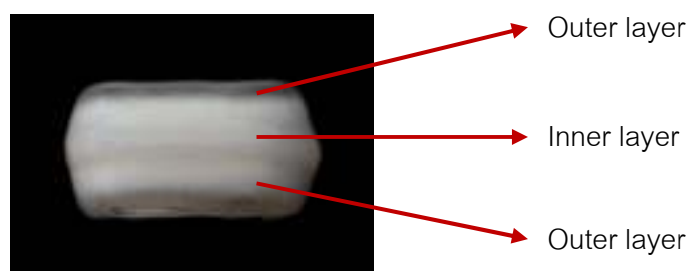
Figure 25 Multilayer sustained release tablet of sodium valproate on exposure to dissolution medium at 6 hours
