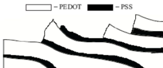
Figure 2.8 The lamellar structure of PEDOT: PSS blend
