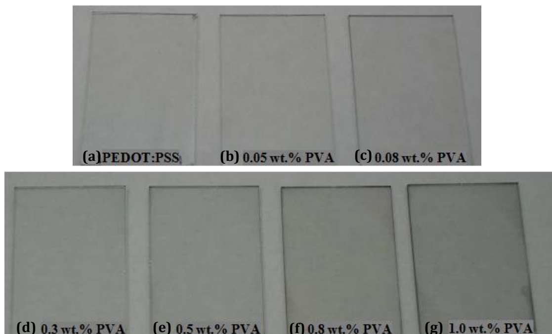
Figure 5.2 (a) PEDOT:PSS thin films on glass slides with various wt.% PVA, (b) 0.05, (c) 0.08, (d) 0.3, (e) 0.5, (f) 0.8, and (g) 1.0
