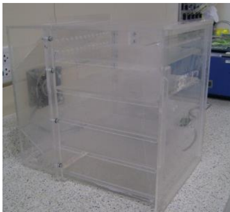
Figure A.4 Blower cabinet for film casting and drying
