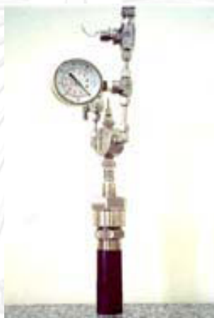
Figure 3.1 Micro-reactor volume of 70 ml
