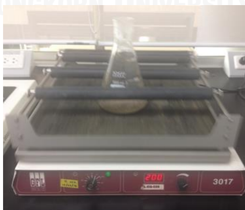
Figure 3.8 Dolomite sorbent was shaken on rotary shaker at 200 rpm
