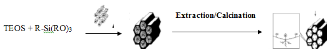
Figure 2. 4 Co-condensation method for the organic modification of mesoporous pure silica phases, R= organic functional group
