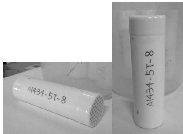
Figure 3. 5 Ceramic membrane with pore size diameter of 0.1 \mu\text{m} .
