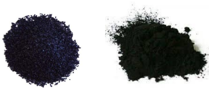
Figure 2. 4 Types of activated carbon: GAC (left) and PAC (right).
