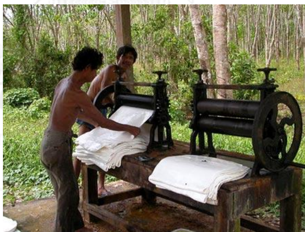
Figure 2.4 Milling which is done by passing coagulum through successive pairs of adjusted rollers [13]
