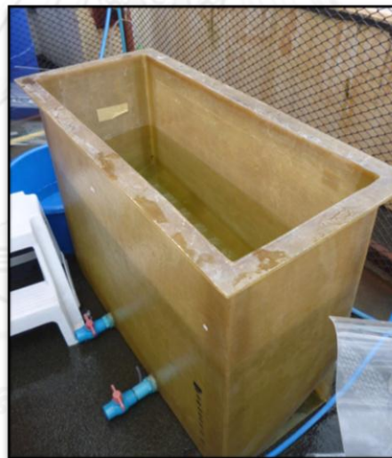
Figure 3.3 Novel non-baffled flat panel airlift contactors
