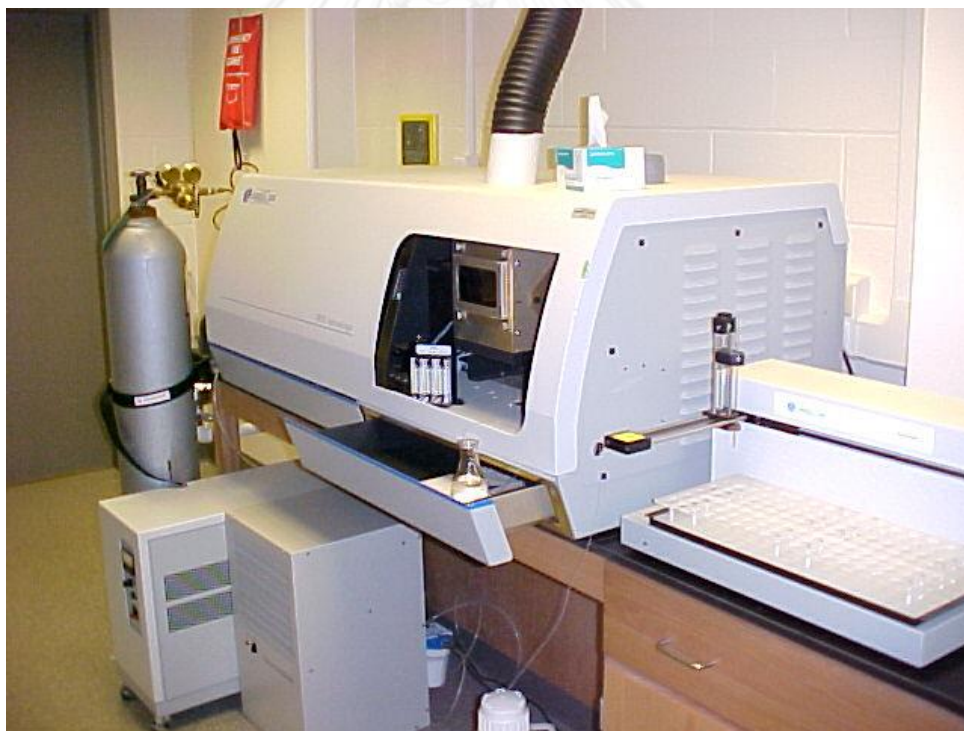
รูปที่ ข.3 Inductively Couple Plasma - Optical Emission Spectrometer (ICP-OES) ("Analytical Instrumentation,")
