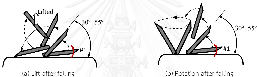
Figure 7.13. Movements of uncoated particles that fell on the lower electrode after departure.
