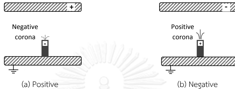
Figure 2.9. Monopolar corona discharge on particles in contact with the lower electrode for different voltage polarities applied to the upper electrode.
