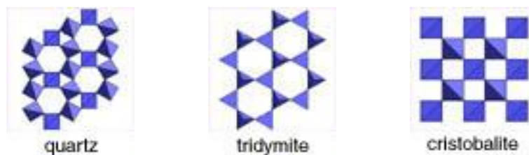
Figure 2. 4 Crystalline structure of silica [14].
