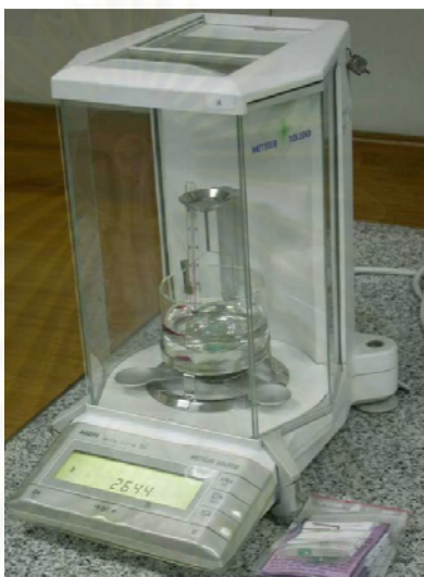
Figure 3.5 Mettler Toledo (model AG204) electronic balance used to weigh and determine specific gravity of coarse-grained samples.
