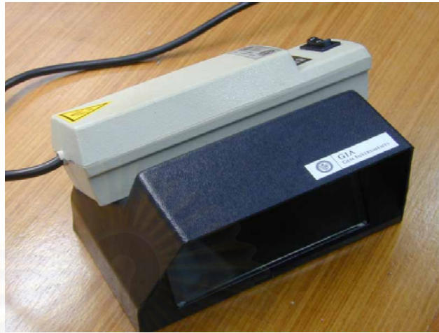
Figure 3.6. Mineralight lamp (UVGL 25) generating both long-wave (365 nm) and short-wave(254 nm) of ultraviolet engaged to observe fluorescence phenomena of the studied olivines.
