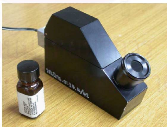
Figure 3.4. A-Kruss refractometer with sodium light source used in this research project.
