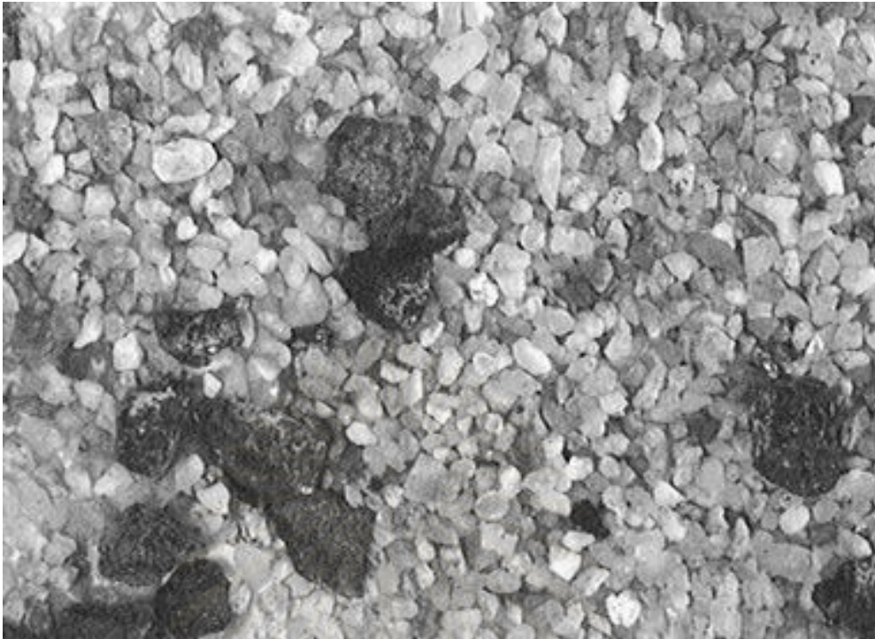
Figure 2.10 Mixed particles between coal and sand after primary fragmentation study at 850 °C, 1 atm with N 2 as the fluidizing gas by CCD camera.
