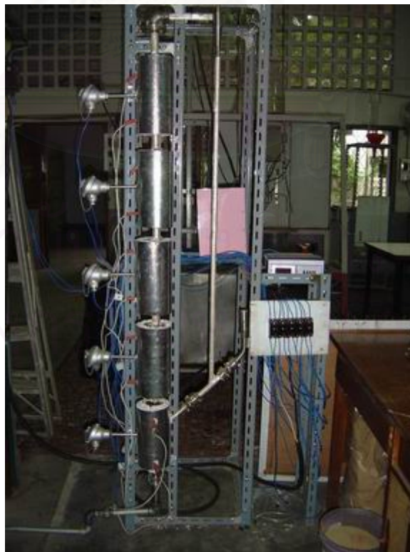
Figure 2.3 CFBC in the experiments.
