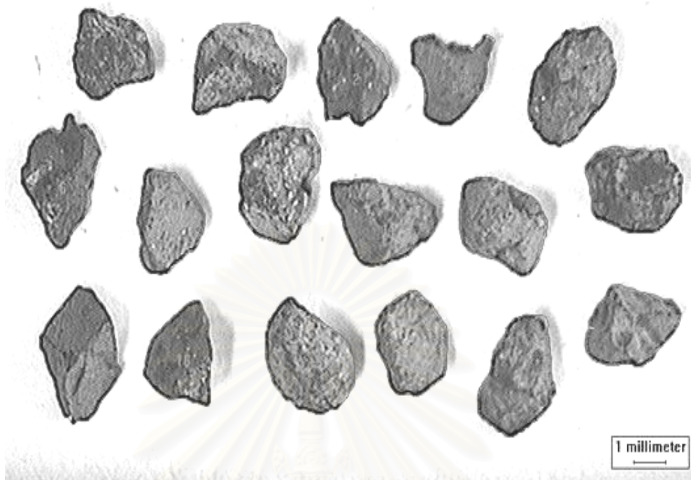
Figure 2.6 Coal particles after attrition at ambient environment that captured by CCD camera and analyzed by Image Pro Plus.
