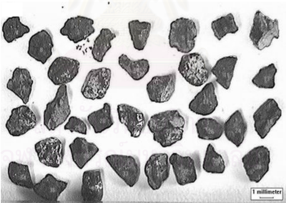
Figure 2.11 Coal particles after primary fragmentation at 850 °C, 1 atm with N 2 as the fluidizing gas that captured by CCD camera and analyzed by Image Pro Plus.
