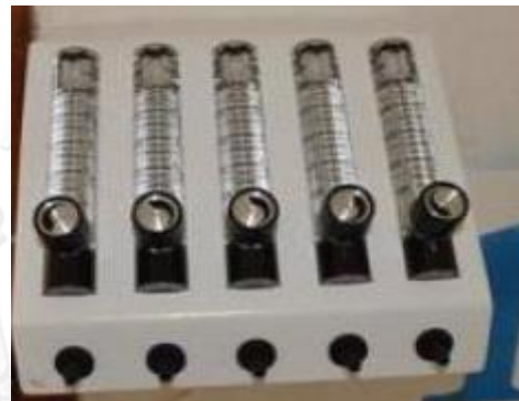
Figure 4 Oxygen Sureflow ( flow splitter)
