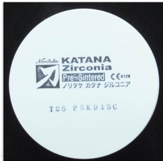
Figure 14 KATANA Pre-Sintered Zirconia Block
