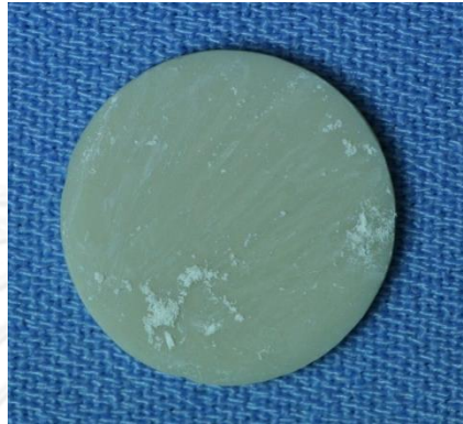
Figure 50 The white powder coated on HF-treated zirconia surface without ultrasonic cleaning
