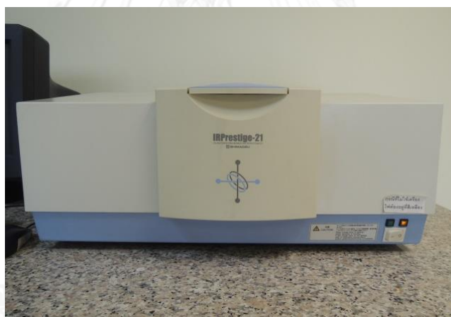
Figure 19 Fourier Transform Infrared (FTIR) spectrometer
