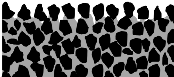
Figure 59 Drawing picture demonstrates lateral view of dental porcelain surface, composing glassy matrix (gray color) and crystal grains (dark color) with the average particle size in micrometer scale.
