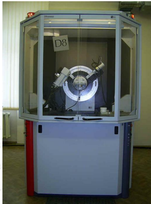
Figure 20 The diffractometer for XRD analysis
