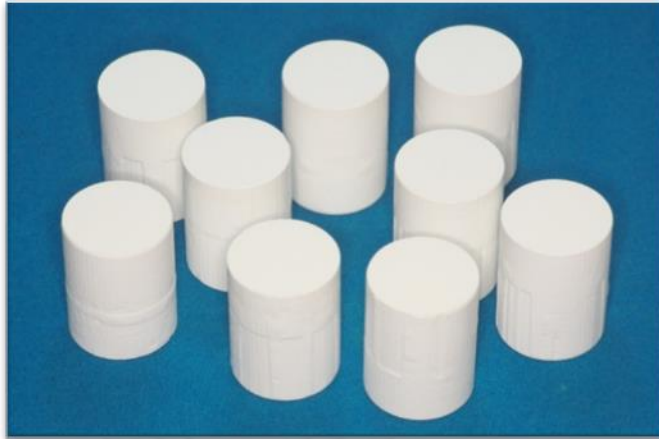
Figure 16 The cylinder-shaped of the pre-sintered zirconia ( \varnothing ~19 mm, height ~21 mm).
