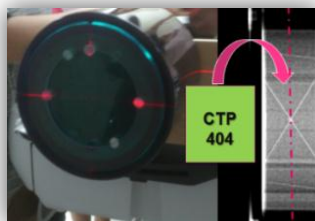
Figure B 9 Catphan phantom setting and reference line of CTP 404 section. (Slice width, sensitometry and pixel size module).
