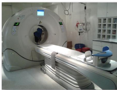
Figure 3.3 The 320-row MDCT (Aquilion ONE, Toshiba Medical Systems Corporation, Japan) scanner.
