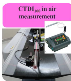
Figure 4.1 CTDI 100 in air ( C_{air} or CTDI air ) measurement using pencil ion chamber set in air, at isocenter of CT gantry bore.
