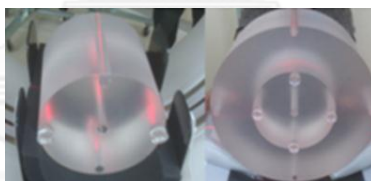
Figure 3.4 Two sizes of standard cylindrical PMMA head (16 cm in diameter) and body (32 cm in diameter) CT dosimetry phantoms with holes for acrylic rods insertion at various location of the hole.
