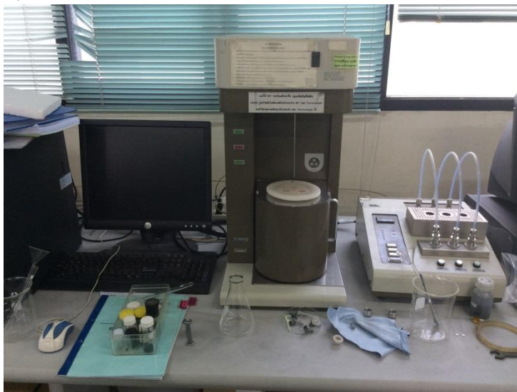
Fig. 13 Automatic specific surface area/pore size distribution measurement (BELSORP-mini II, BEL JAPAN INC).
