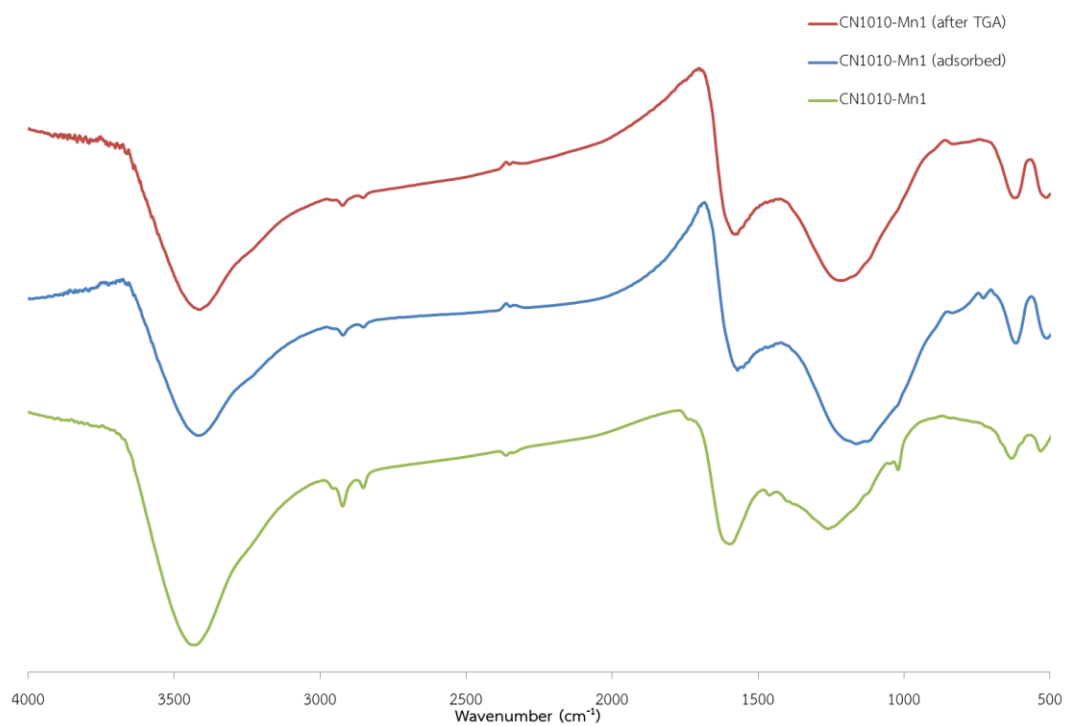
Fig. 29 (g) FTIR spectra of CN1010-Mn1
