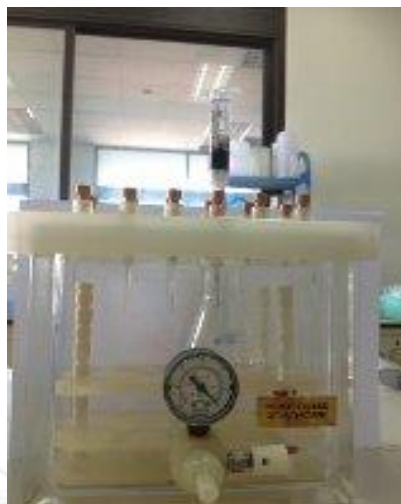
Figure 3.1 Photograph of cylinder column extraction setup.
