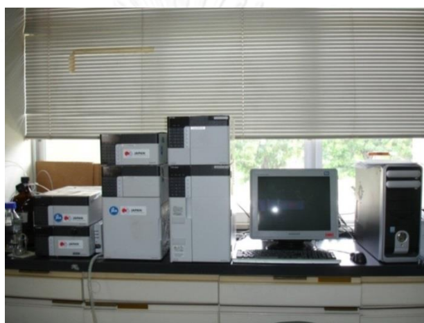
Figure 3. 14 A High Performance Liquid Chromatography with UV-VIS detector, model Shimadzu SPD 20A, Japan
