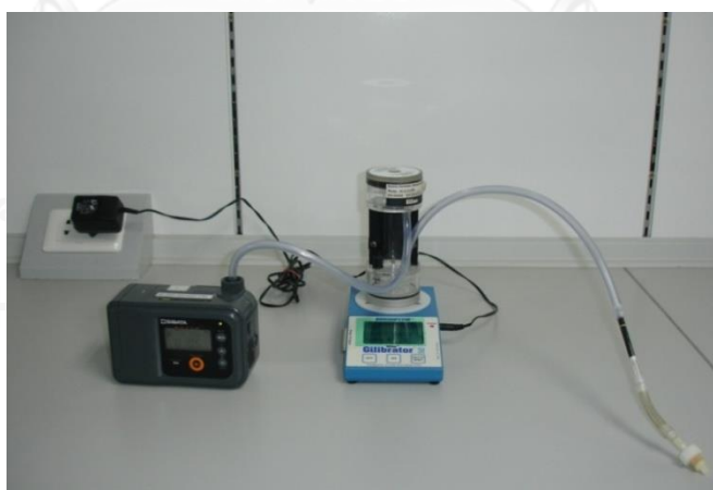
Figure 3. 23 Calibration of person air pump by using bubble gas calibrator
