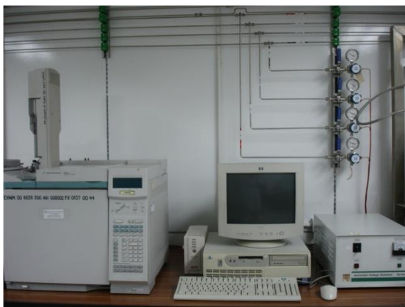
Figure 3. 15 Gas Chromatography with flame ionization detector, Agilent Technology model HP 6890N, USA
