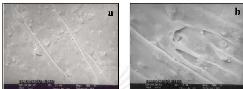
Figure 2.8 SEM micrographs of LDPE/starch blown film a) LDPE/starch (70/30) and b) LDPE/starch (50/50) [7]
