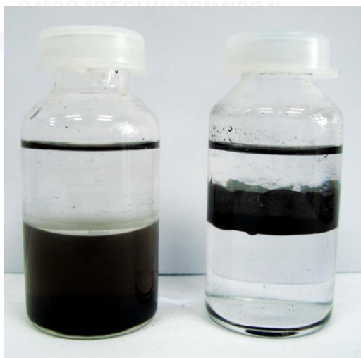
Figure 4.12 Dispersion of GO (left) and GO-alkyne (right) in water/hexane (0.5 mg/ml)
