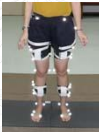
Figure 3.15 shows the IMU devices and the reflective markers that are placed on the participants.
