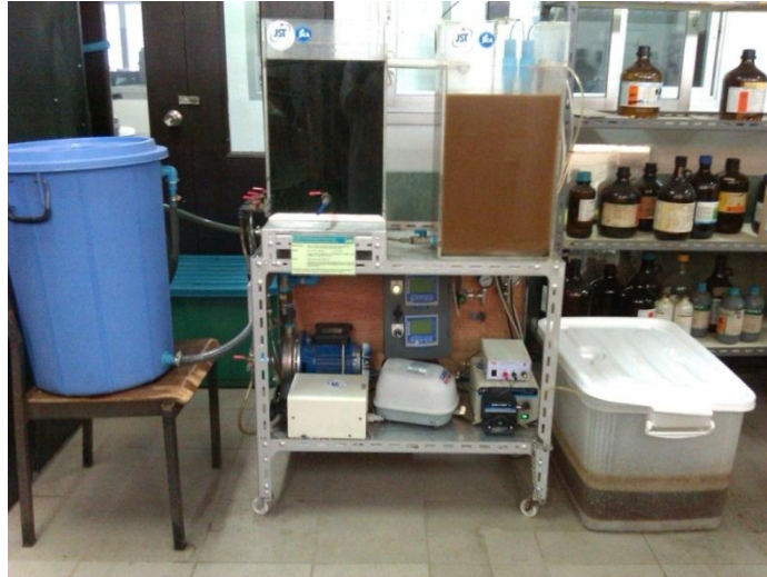
Figure A.3 Configuration of Laboratory-scale it-MBR at Kasetsart University.
