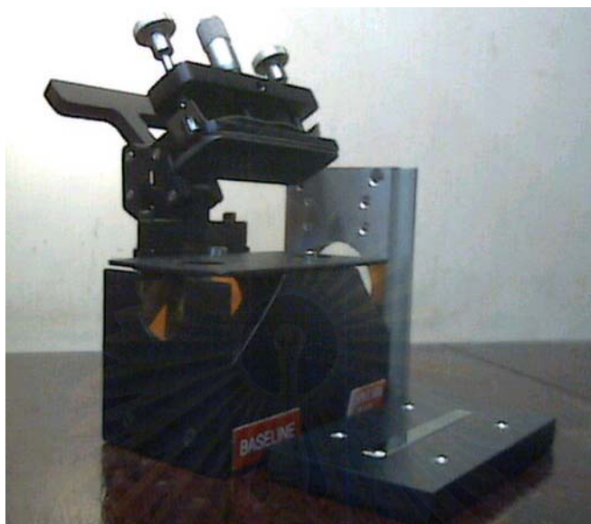
Figure 4.2 Photograph of the Baseline HATR equipped with Single-pass trapezoidal germanium plate
