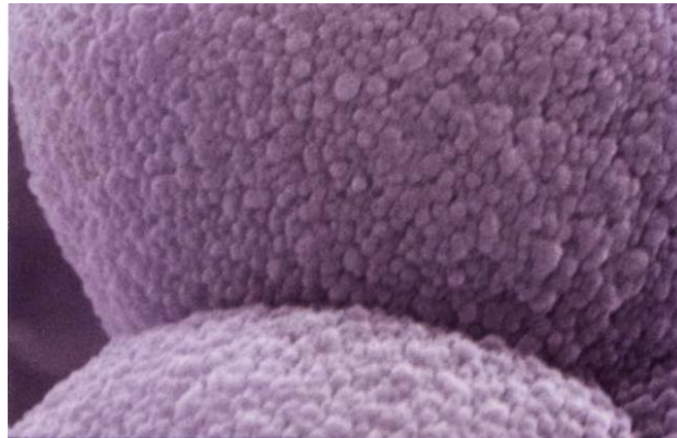
Figure 2.4 SEM image of the magnified vaterite particles
