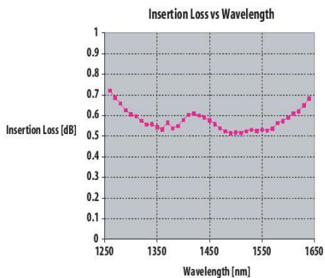
Figure 1: Example of insertion loss of the MAP Variable Optical Attenuator with single-mode fiber
