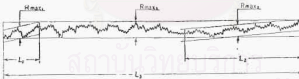
Fig. 1. Determination of the Maximum Height from the Selected Parts of a Profile Curve
