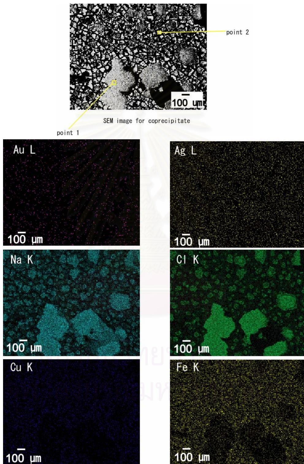
Figure 5.8 SEM image and distribution of metal hydroxide (on the filter paper) after co-precipitation at pH 6, reaction time 1 hour, room temperature.
