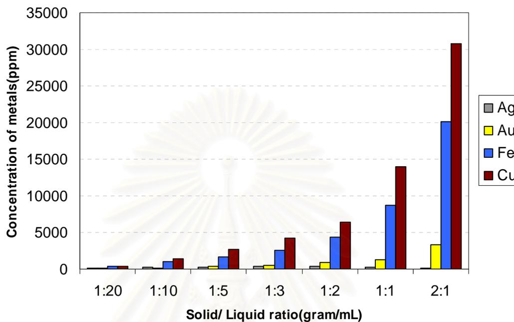
Figure 4.5 Metal concentration in the leachate as a function of ratio sample: aqua regia; reaction time 1 hr., volume of aqua regia 100mL.
