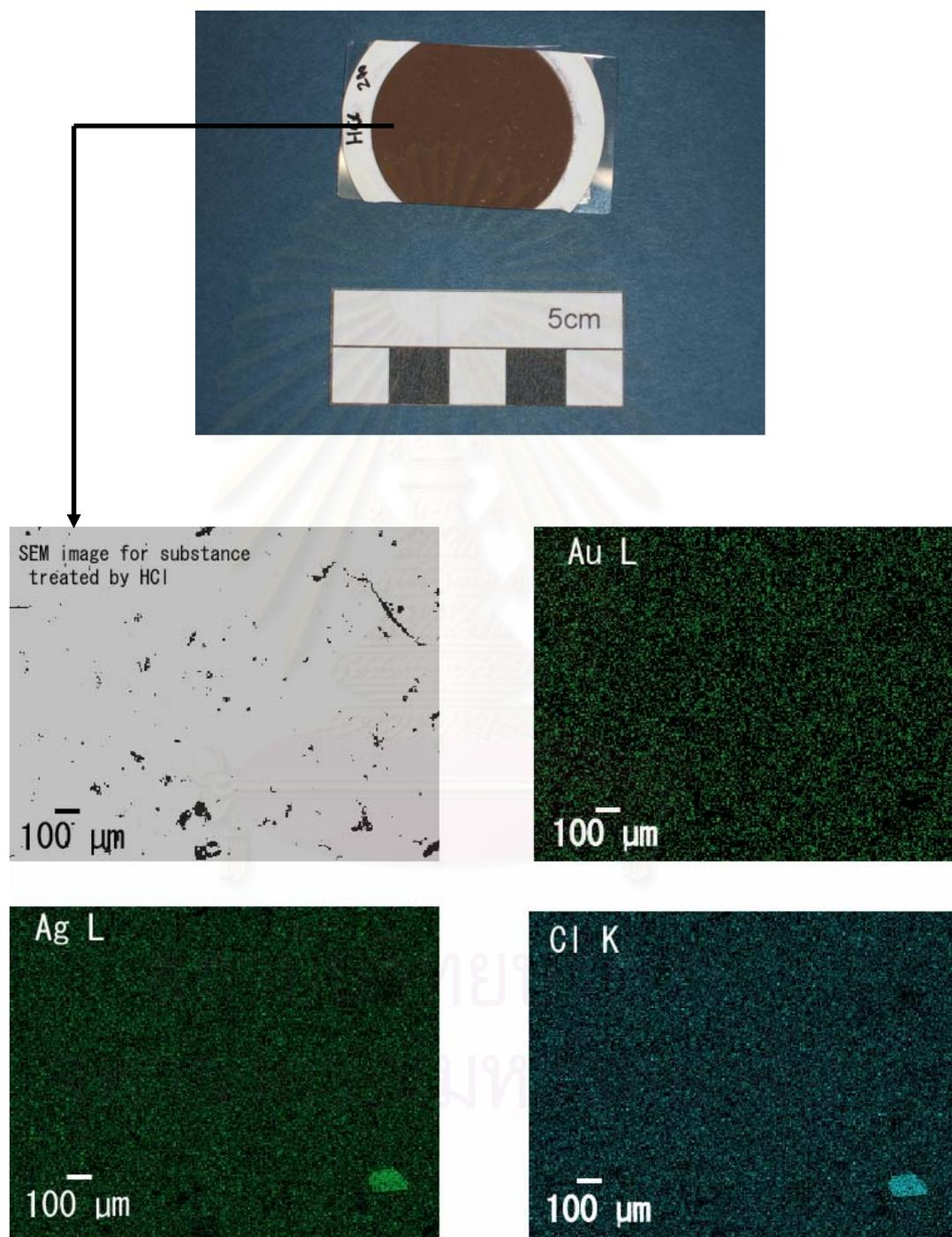
Figure 5.12 SEM image and distribution of the residue (on the filter paper) after purification by 1M HCl. 50 ml. reaction time 1 hour, at room temperature.
