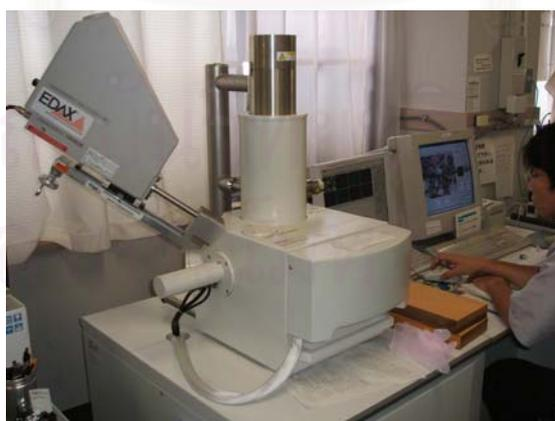
Figure A-12 Shimadzu Superscan SS-550 scanning electron microscopy (SEM-EDX) at the Analytical center, Kyushu University, Japan.
