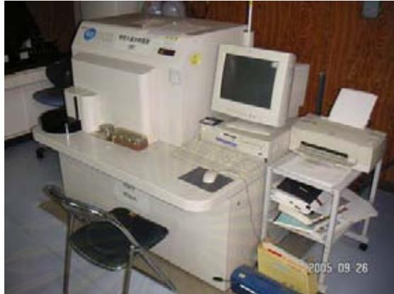
Figure A-2 Rigaku RIX 3100 X-ray fluorescence spectrometer (XRF) at the Department of Earth Resources Engineering, Kyushu University, Japan
