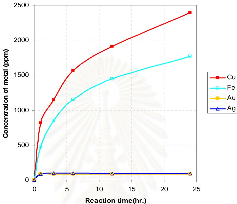
Figure 4.3 Metal dissolution in the leachate as a function of reaction time at room temperature, 5g. of sample(residue after nitric acid parting), 100 mL. of aqua regia
