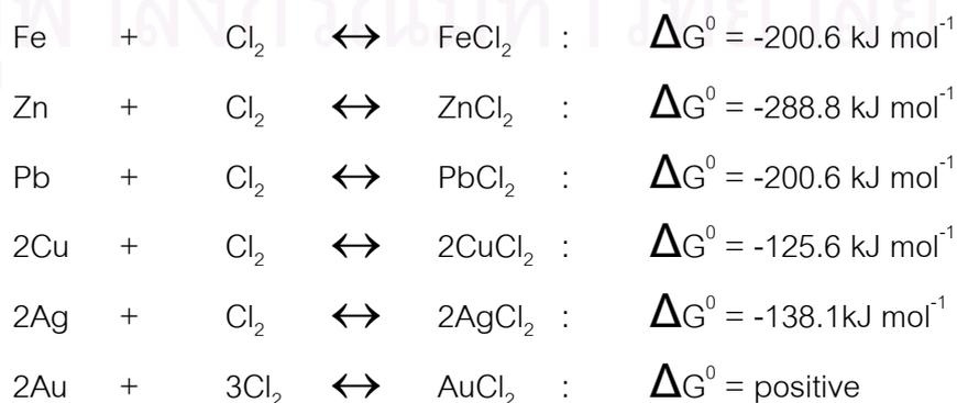
The metals are converted to their respective chlorides in the sequence Fe > Zn > Pb > Cu > Ag >>> Au, as illustrated graphically in Figure 2.6
