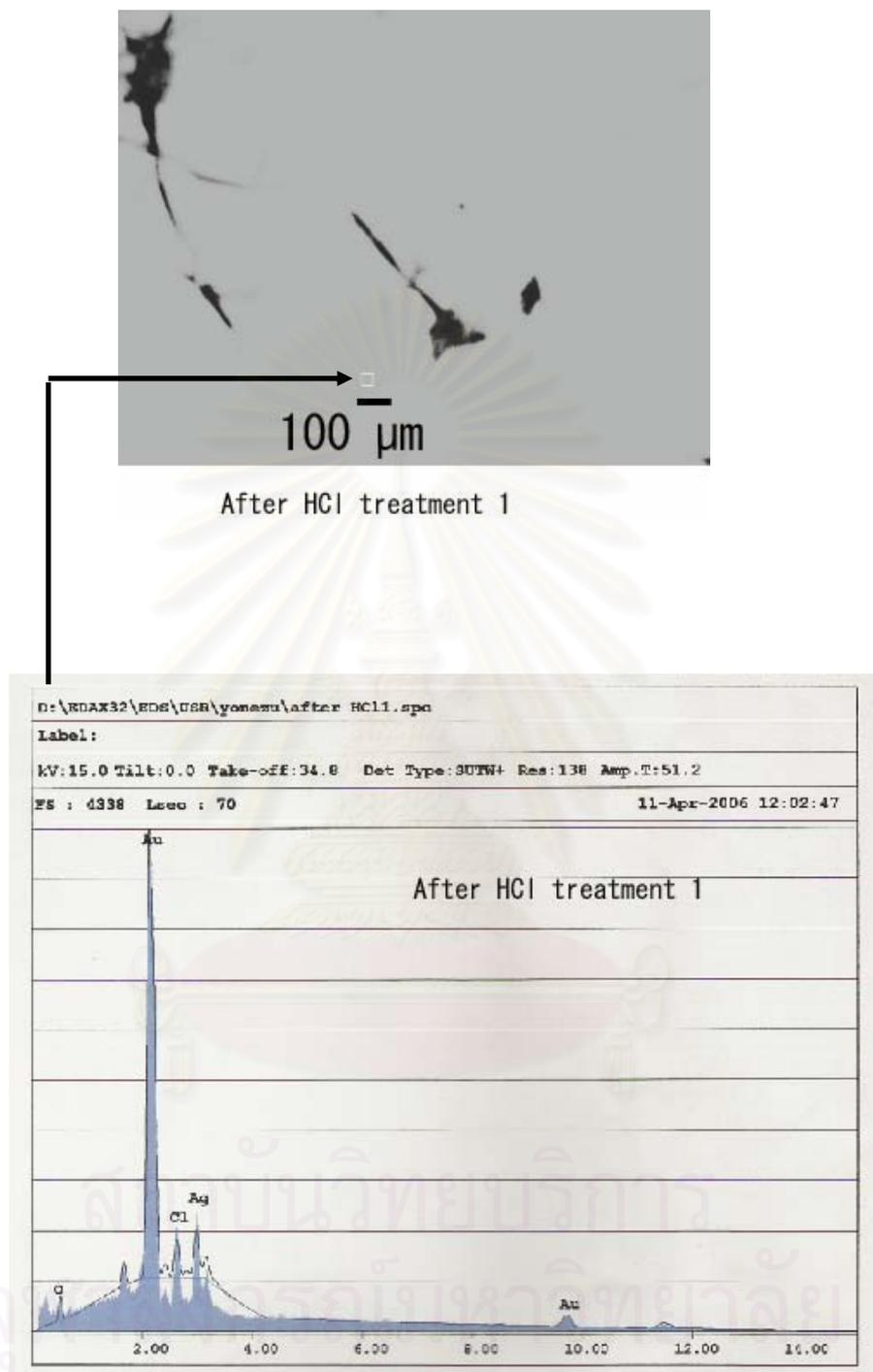
Figure 5.13 The spectrum showing the chemical composition of the residue (on the filter paper) after purification by 1M HCl 50 ml. reaction time 1 hour, at room temperature.
