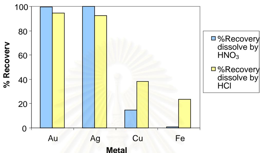
Figure 5.10 Percent of metal recovery after purified with 1M  $\text{HNO}_3$  and 1M  $\text{HCl}$ . 50ml. reaction time 1 hour, at room temperature.
