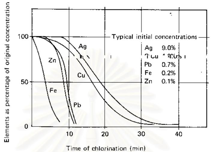
Figure 2.6 The effect of chlorination time on metal removal.
