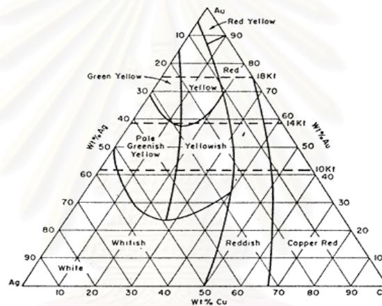
Figure 2.2 Weight percent composition ranges for various colors of Ag-Ag-Cu.
