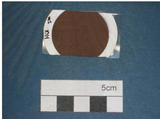
Figure A-11 The samples (on filter paper) fixed on the slide glass for observation by optical microscope.
