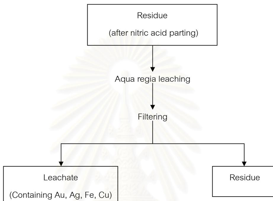
Figure 4.2 Aqua regia leaching experiment procedure used for residue after nitric acid parting.
