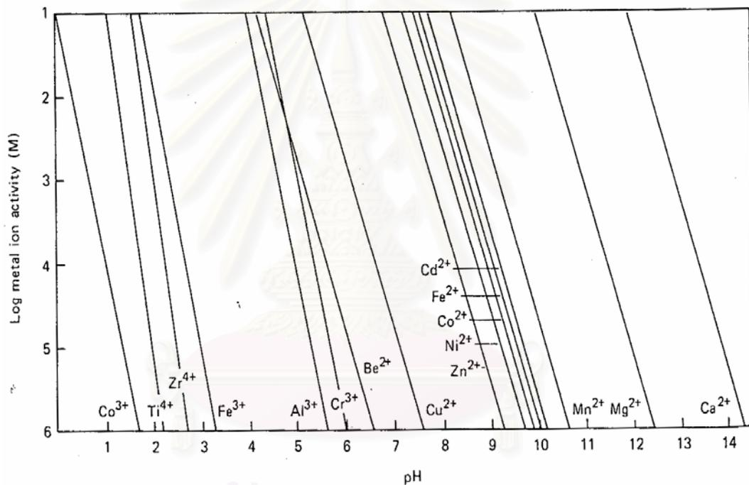
Figure 5.3 Precipitation diagram for metal hydroxides.
