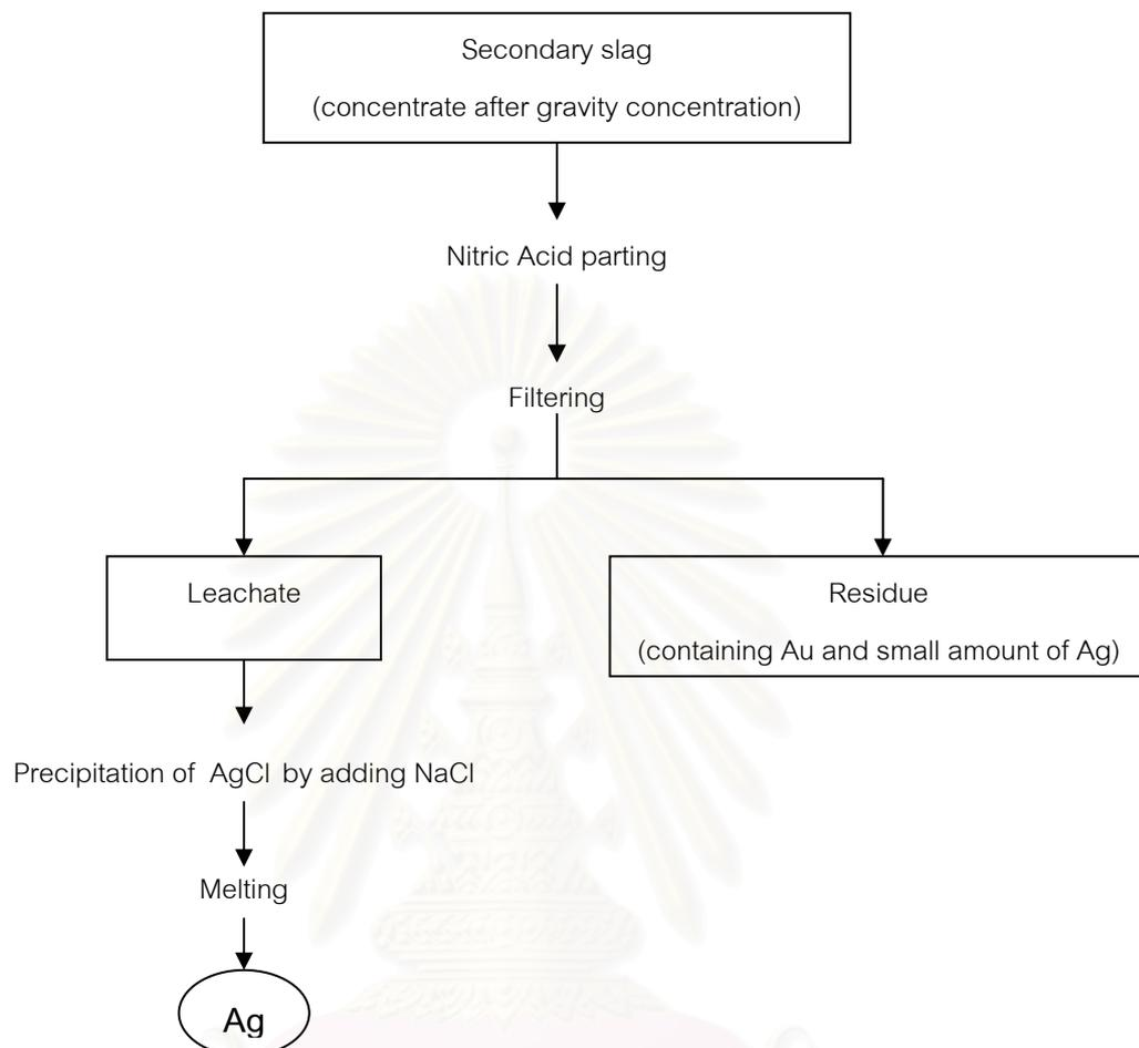
Figure 4.1 Nitric acid parting experiment procedure used for concentrate after gravity concentration.
