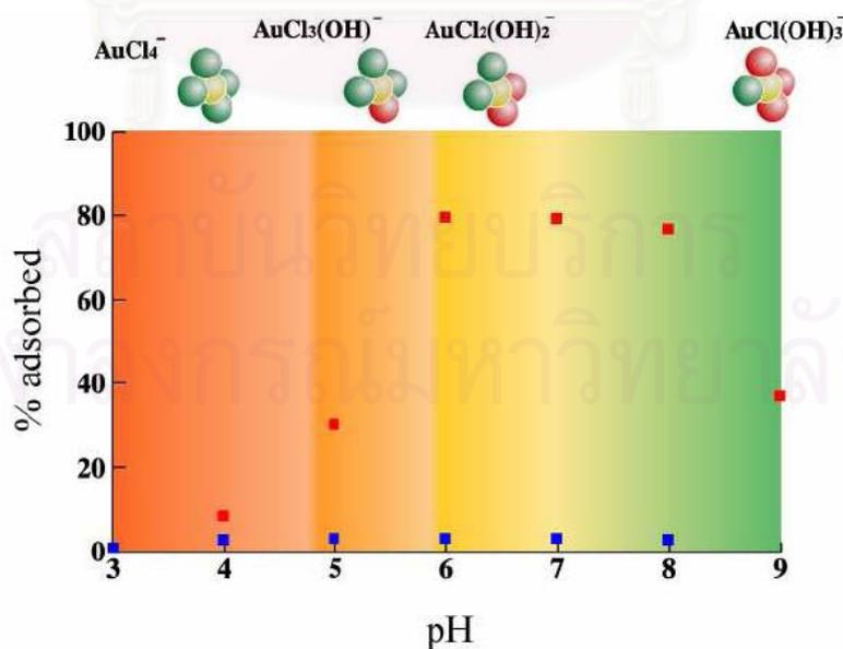
Figure 5.1 The effect of pH on adsorption of gold ions (below) and the pre-dominant gold species in each pH solution. (*Baes and Mesmer, 1976*)
