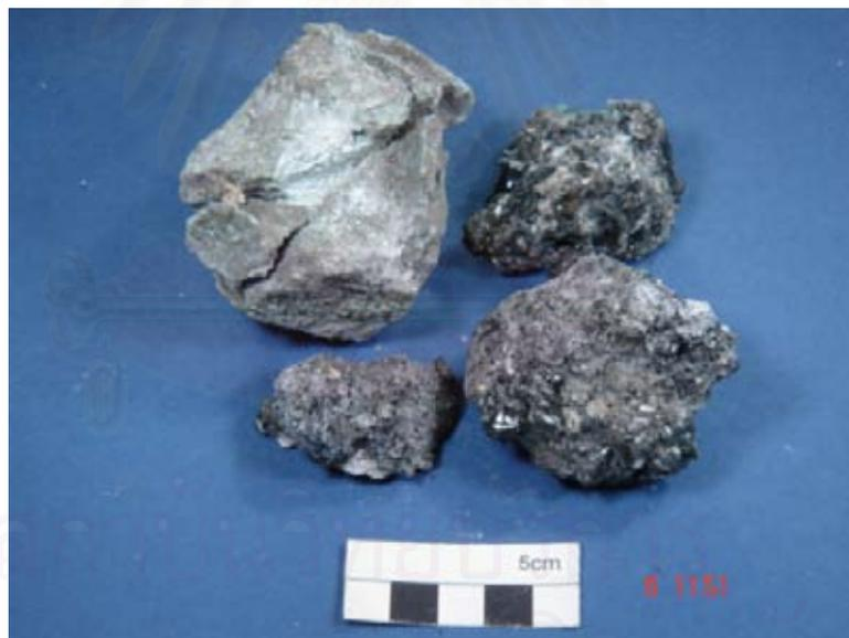
Figure 3.1 Original Secondary slag.
