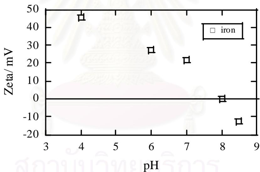
Figure 5.2 Zeta potential for iron (III) hydroxide as a function of pH in  $0.12 \text{ mol dm}^{-3}$  NaCl solution. (Uchida, 2002)
