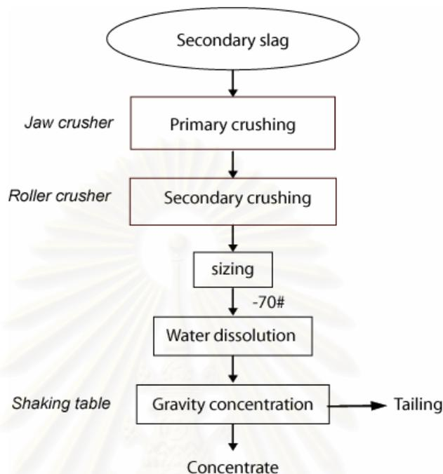
Figure 3.2 Physical concentrations to recovery gold and silver from secondary slag.
