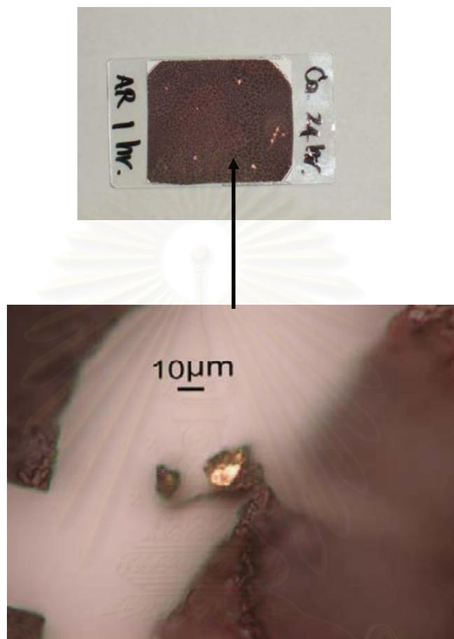
Figure 5.7 Photomicrograph of gold particle on metal hydroxide after co-precipitation at pH 6, reaction time 1 hour, at room temperature.
