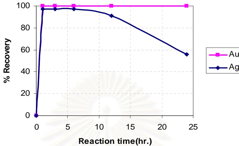
Figure 4.4 Percent recovery of gold and silver as a function of reaction time at room temperature, 5g. of sample(residue after nitric acid parting), 100 mL. of aqua regia.(Calculated from XRF result data of residue after leaching experiments from Table 4.3)
