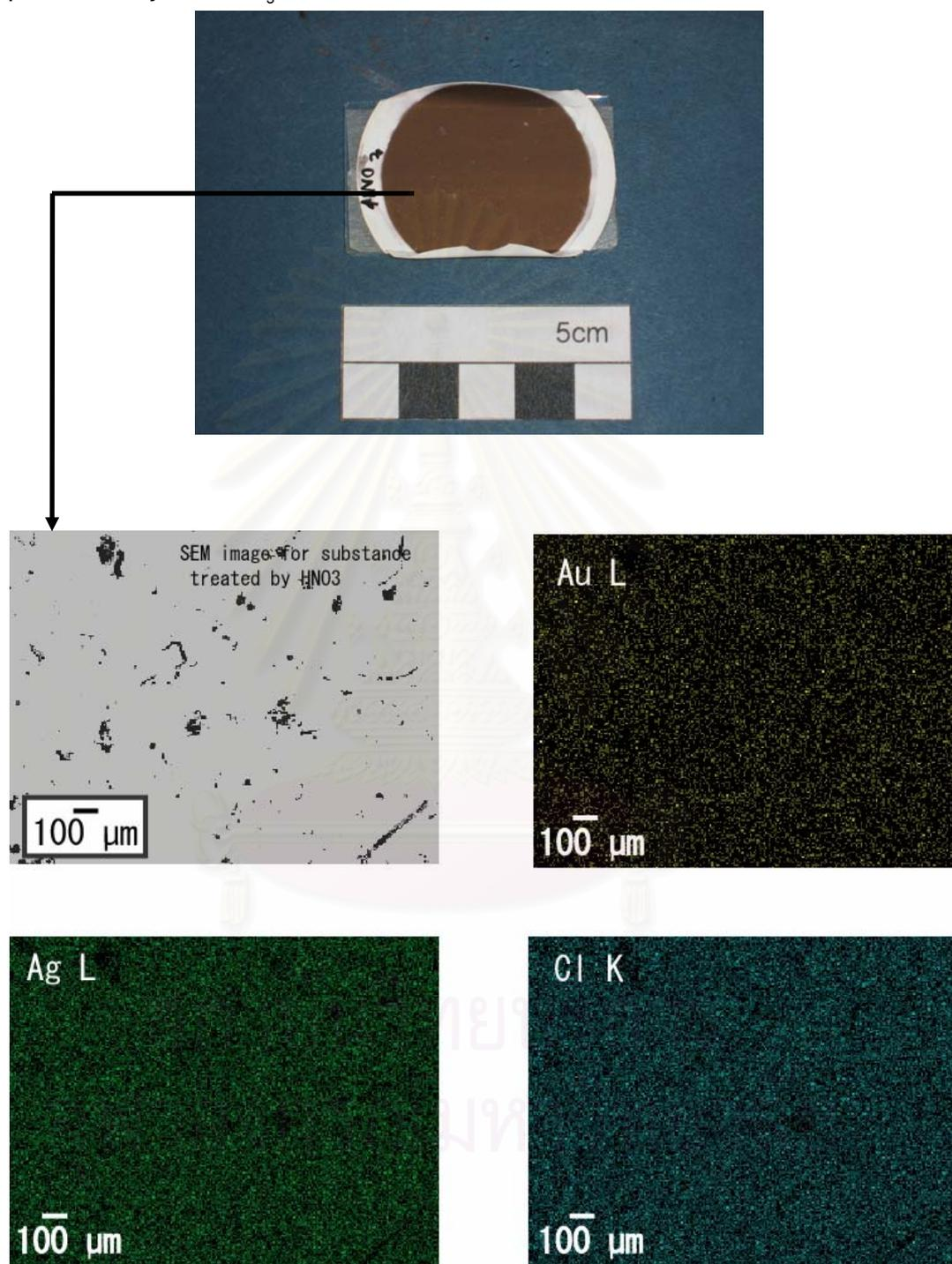
Figure 5.14 SEM image and distribution of the residue (on the filter paper) after purification by 1M  $\text{HNO}_3$  50 ml. reaction time 1 hour, at room temperature.
