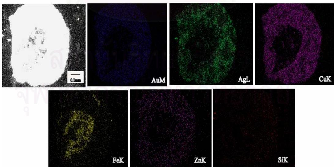
Figure 3.4 SEM photograph and X-ray images for AuM $\alpha$ , AgL $\alpha$ , CuK $\alpha$ , FeK $\alpha$ , ZnK $\alpha$  and SiK $\alpha$  of metallic particles in the concentrate after gravity concentration.
