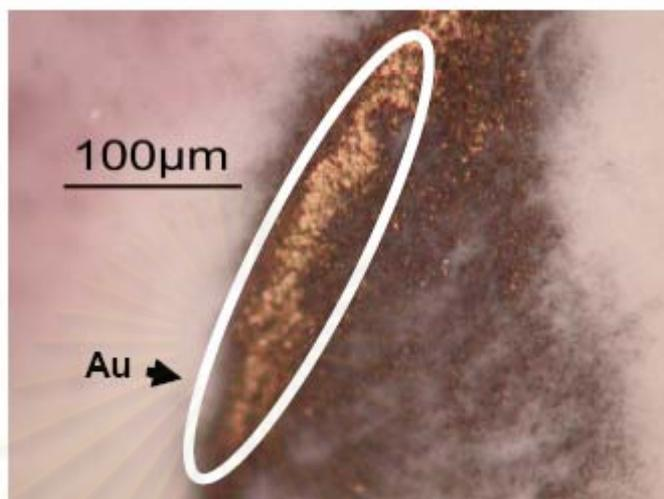
Figure 5.11 Photomicrograph of gold particle after purification by 1M HCl. 50 ml. reaction time 1 hour, at room temperature.
