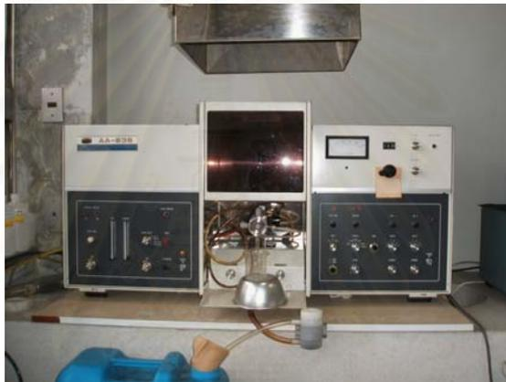
Figure A-7 NIPPON Jarrel Ash AA-835 flame atomic absorption spectrophotometer (AAS) at the Department of Earth Resources Engineering, Kyushu University, Japan
