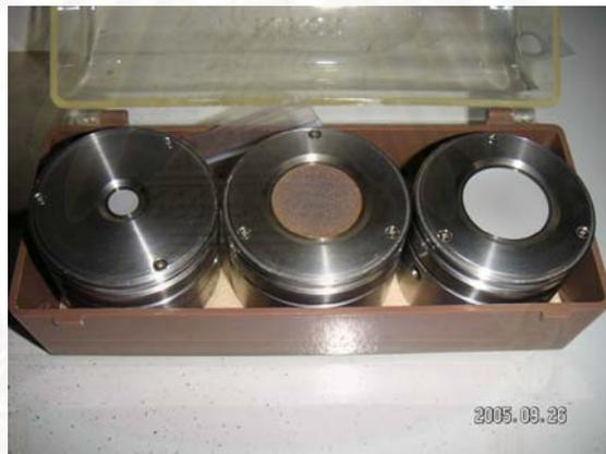
Figure A-3 Standard samples for analyze XRF
