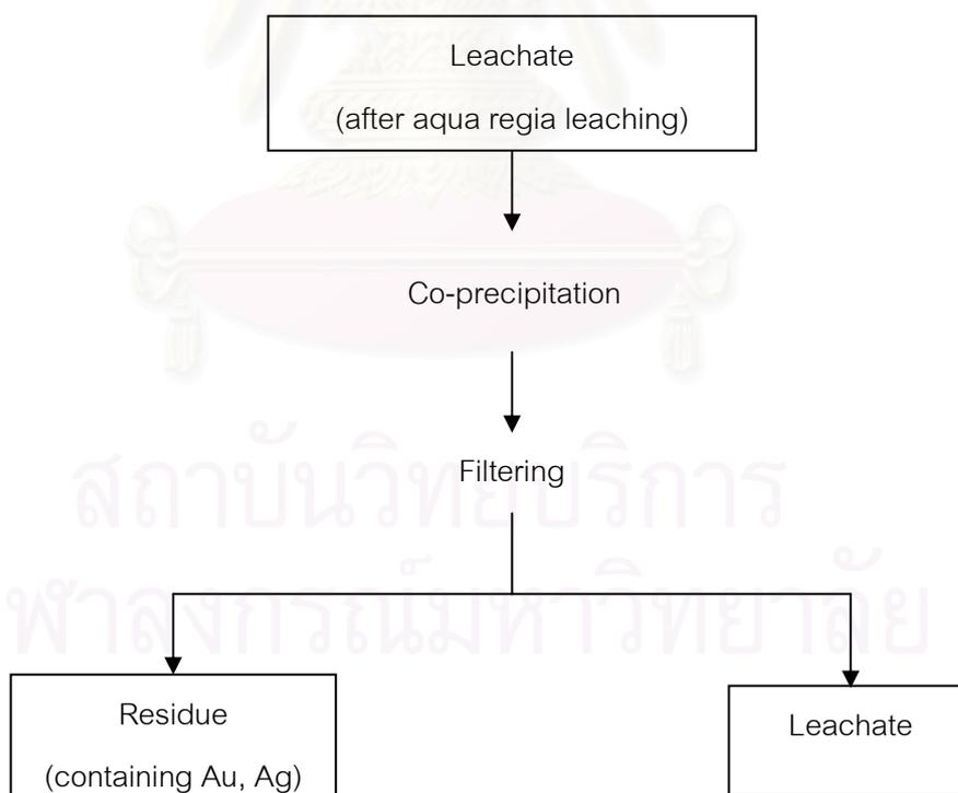
Figure 5.4 Co-precipitation experiment procedure used for leachate after aqua regia leaching.
