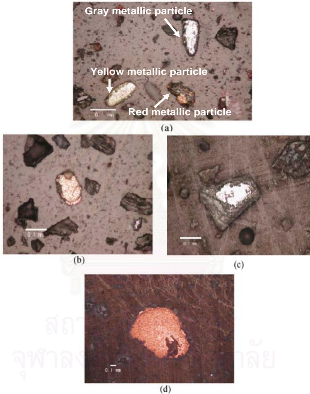
Figure 3.3 Photomicrographs of the concentrate after gravity concentration.
