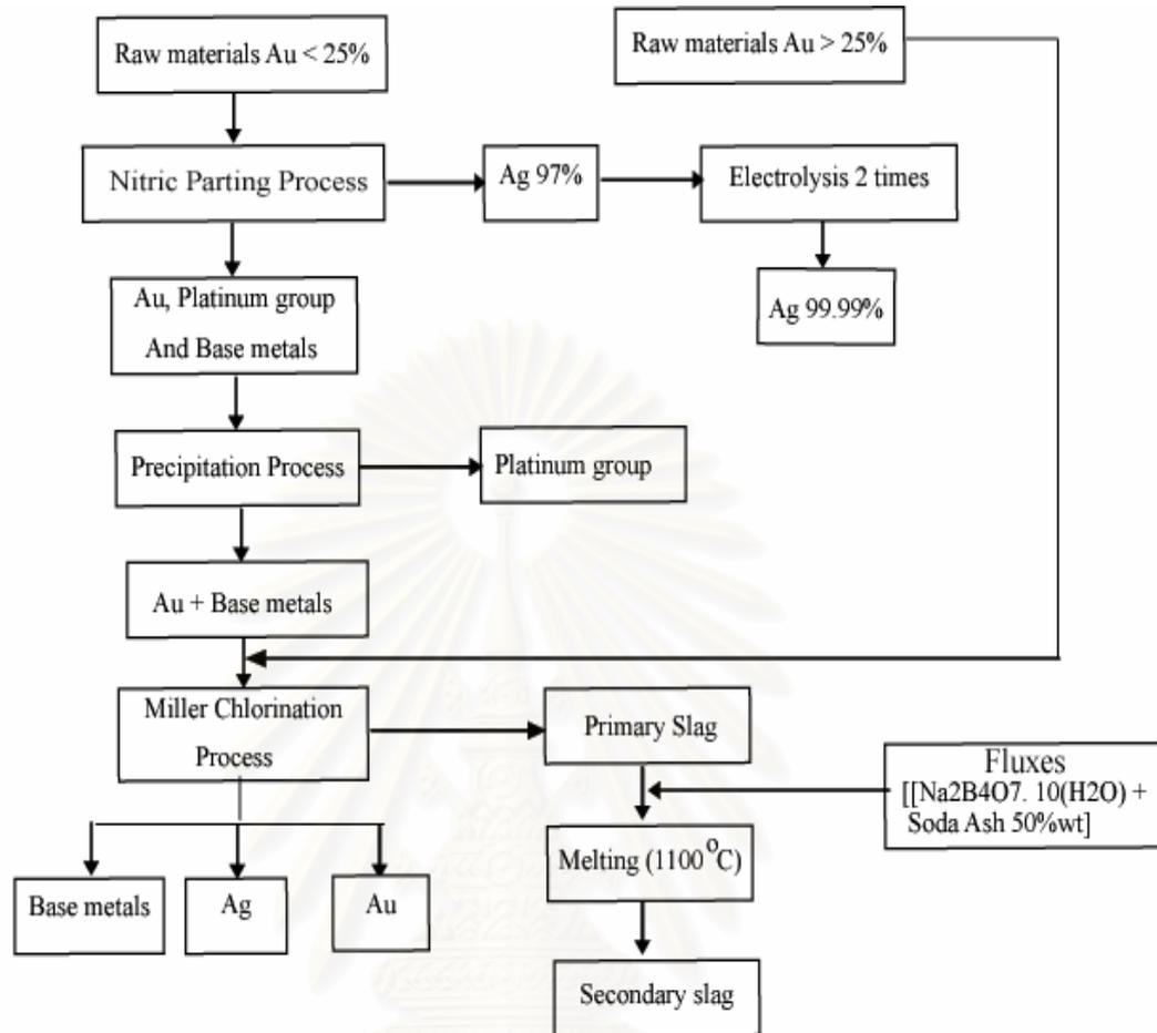
Figure 1.2 Flowchart of gold refining process.
