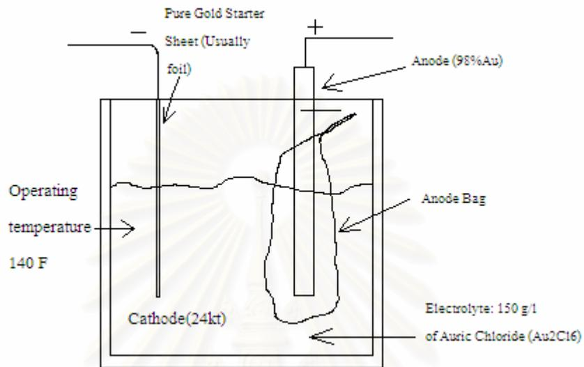
Figure 2.7 Basic gold electrorefining cell (Wohlwill cell).
