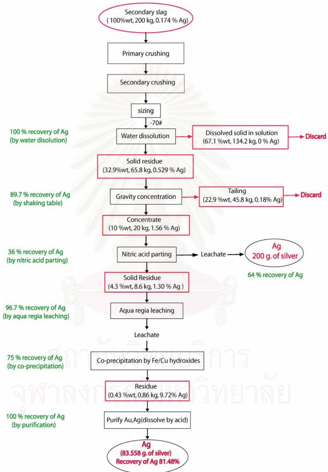
Figure 6.2 Variation of the total amount of secondary slag and silver concentration in all stages of the recovery process.
