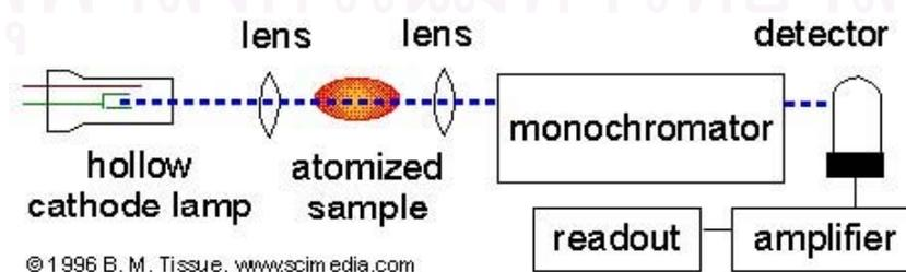
Figure A-6 Schematic of an atomic-absorption experiment
