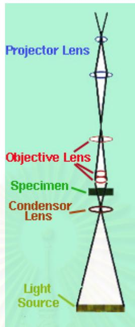
Figure A-8 Schematic diagram of the optical micrograph
