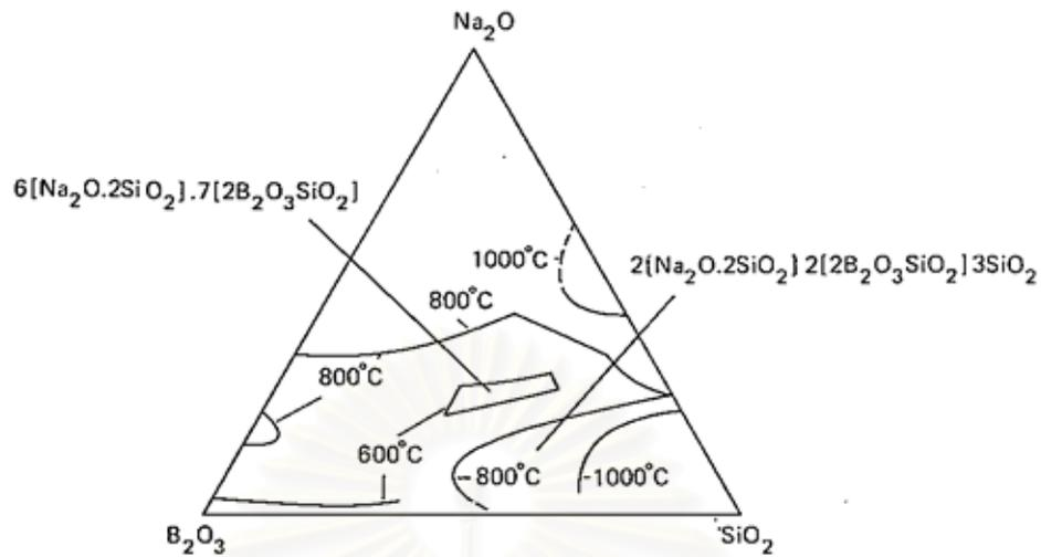
Figure 2.9  $\text{Na}_2\text{O} - \text{B}_2\text{O}_3 - \text{SiO}_2$  phase.
