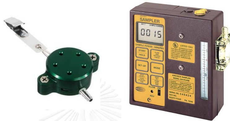
Figure 9 PM 10 personal monitor equipment
