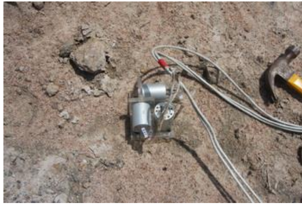
Figure 12 2.0-Hz triaxial geophone
