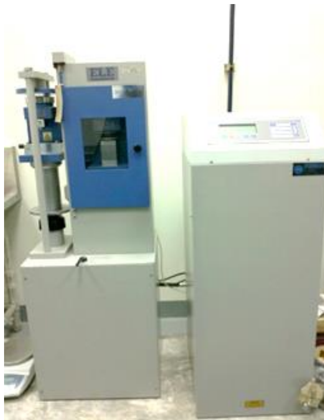
Figure 3.2 Concrete Compression Machine
