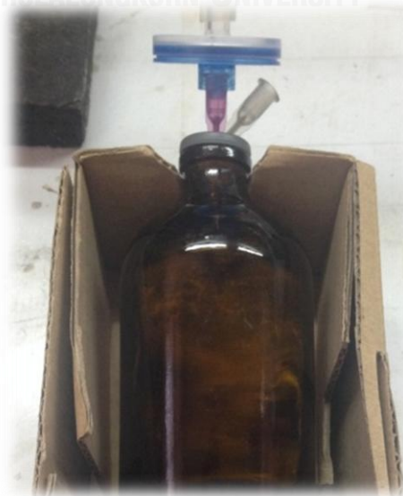
Figure A.5 Purging nitrogen gas
