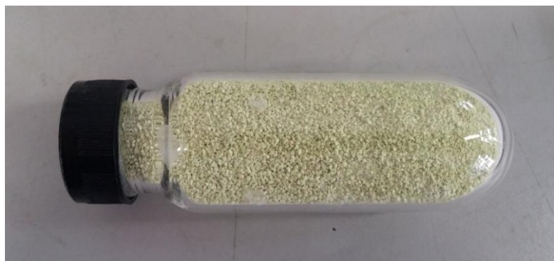
Figure 4.1 synthesized iron molybdate
