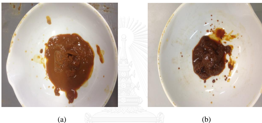
Figure 4.23 Concentrated iron sludge from centrifugation (Fenton process operated at 100 mg/l initial oil concentration, \text{Fe}^{2+} = 50 mg/l and \text{Fe}^{2+}/\text{H}_2\text{O}_2 ratio= 1:2.5) (a) reuse time = 0, (b) reuse time = 4
